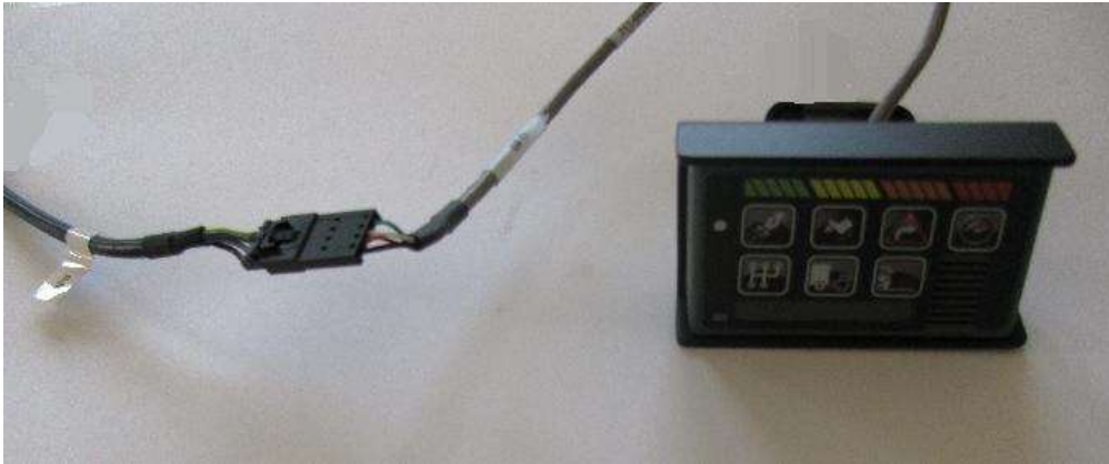
Figure 26: Connecting the DFD Cable to the DFD Thread of the Cello Harness
